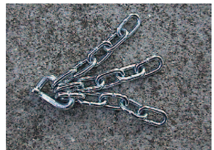
The heart of the tiedown: three sets of five links of 3/16-inch proof chain with a 5/16-inch repair link.
